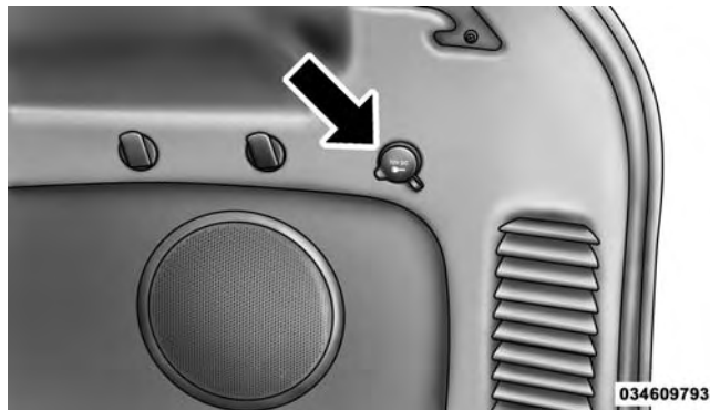
Rear Power Outlet
