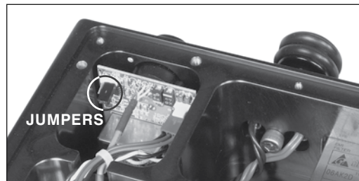
FIGURE 1: Location of Jumper J103 on the inside back panel of the Model 501
