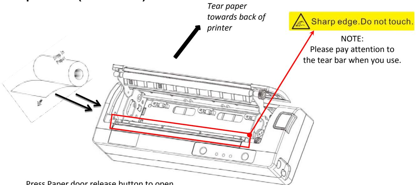
Press Paper door release button to open the paper compartment door. Pull small leader of paper out and close paper door. “Clicks” when properly closed.
