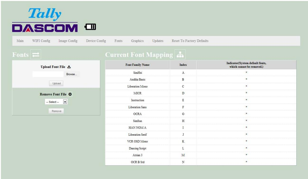
The screenshot displays the Tally DASCUM web interface for font management. The navigation bar includes: Main, WIFI Config, Image Config, Device Config, **Fonts**, Graphics, Updates, and Reset To Factory Defaults. The 'Fonts' section is active, showing two main areas:
