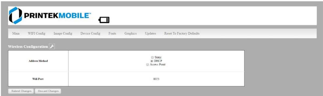
The screenshot shows the Printek Mobile web interface. At the top is the Printek Mobile logo and a navigation menu with links: Main, WIFI Config, Image Config, Device Config, Fonts, Graphics, Updates, and Reset To Factory Defaults. The main content area is titled "Wireless Configuration" and contains a table with the following configuration options:
