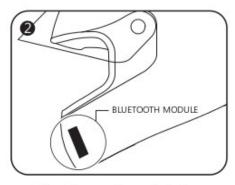
**2** The Bluetooth module has been installed into the helmet behind the front vent.
