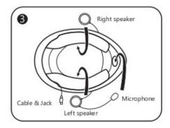
**3** Feed cords under the helmet liner if possible and as close to the bottom of the helmet
