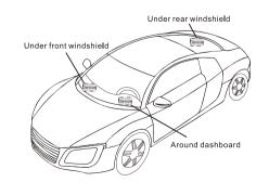
1) The device should face up to the sky. 2) Metal thermal barrier or heating layer of the windshield affects the signal.
