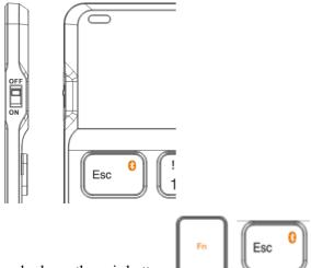
Press and release the pair button + when the "power" LED start to flash blue, the keyboard enters pairing mode.
