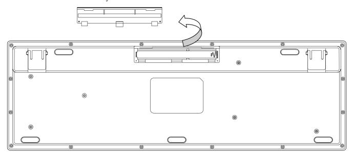
b. Install the battery and match the code
