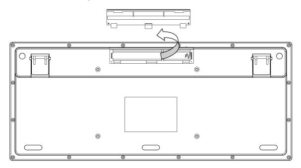
b. Install the battery and match the code
