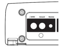
The A6450's "+12 VDC" and "Ground" connections are designed to accept 4 AWG power wire. 4 AWG is a minimum power wire size for this amplifier.
