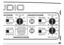
1) "Filter Mode" Control: The A6450 employs a 12dB per octave filter for each pair of channels (one filter for channels 1&2, another filter for channels 3&4 and a third filter for channels 5&6). Each of these filters can be configured independently into one of two filter types or defeated completely by way of the three-position "Filter Mode" switches:
