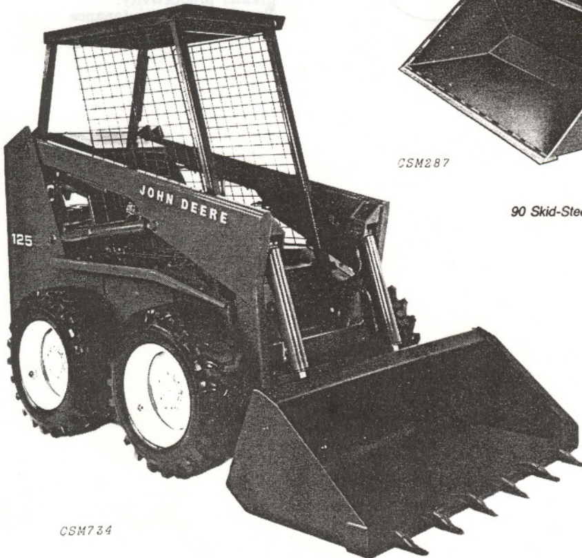
125 Skid-Steer Loader with dirt and foundry bucket and teeth
