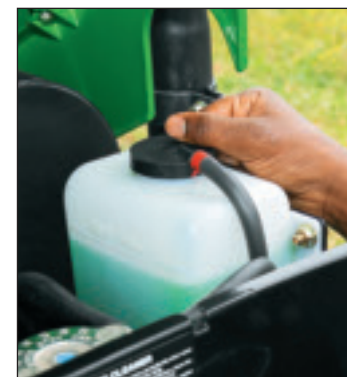
With this translucent coolant reservoir (similar to the one in your car) you can check coolant levels at a glance.
