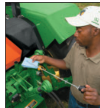
Checking oil levels is easy too. The fluid fills and dipsticks for hydraulic and transmission oils are located near the hitch in an easy-to-reach position.
