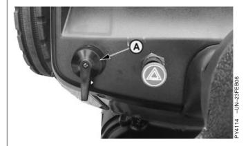
Move turn signal lever (A) down to indicate left-hand turn or up for right-hand turn. Indicator lights (D) will flash to signal turn direction.
