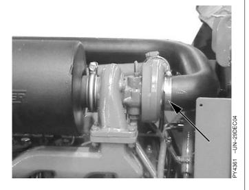
Check all air intake system clamps for tightness.
