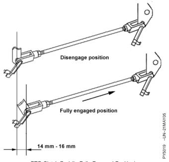
PTO Clutch Rod (In Fully Engaged Position)
