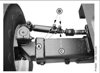
A-Lock Nuts **B**—Tie Rod Bolts C-Inner Tube
