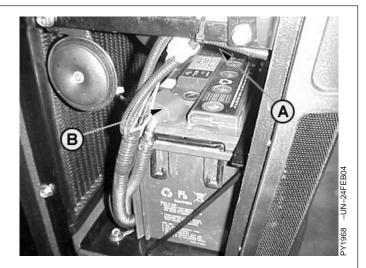
A-Positive (+) Battery Terminal B-Negative (-) Battery Terminal
