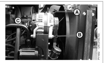
A—Tension Adjustment Cap Screw
