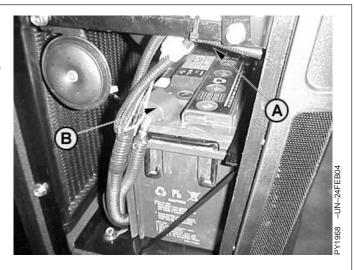
A—Positive (+) Cable Nut B—Negative (—) Cable Nut
