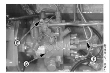
E—Electric fuel shut-off F—Fuel injection lines
