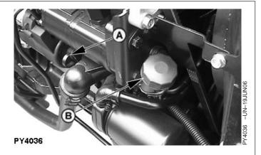
A-Engine Oil Dipstick **B**—Engine Oil Filler Cap
