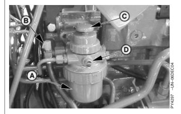
A—FuelGardä fuel filter B—Fuel shut-off valve
