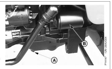
A—Engine Oil Drain Plug
