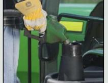
Fuel fills are easy. A new 350-gal. capacity on 4-wheel-drives means you can stop less often to fill up. Capacity on tracks models is now 330 gal.
