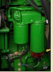
New self-priming fuel system eliminates messy hand priming and filter pre-filling for fast, easy filter changes.
