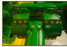
(4) Heavy-duty reaction arm (above) attaches to rear axle and pivots up and down.
