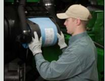
**Annual air filter replacements** are a breeze for all 9030 Series tractors. Filters can be conveniently reached while standing on the ground.
