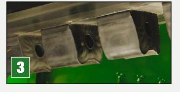
A new 60-degree drive wheel pattern (right) grips the track belt more efficiently, reducing slippage for better performance.
