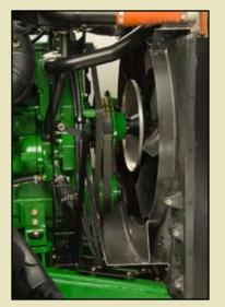
Field-proven Vari-Coof™ system with variable-speed fan drive automatically adjusts its speed to keep the engine and hydraulic system cool. It also improves fuel economy and boosts pulling power.
