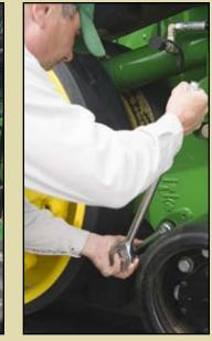
A new toolbox is built into the platform (left) for easy access and for storage of tools, chains, or other equipment. **New track-alignment mechanism** (right) makes adjustments easier and improves belt tracking.
