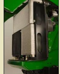
**New radiator** is 29 percent larger than previous models for increased cooling capacity.
