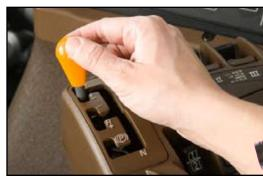
The convenient shift lever on the CommandARM console lets you smoothly move through 18 forward or six reverse gears with just your thumb. Easily shift into park, neutral, forward, or reverse, as well as change gears up or down. Transport up to 24 mph (4WD).
