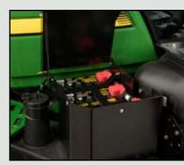
Flip-up battery cover features an air cylinder to hold it up during periodic inspections or annual service.
