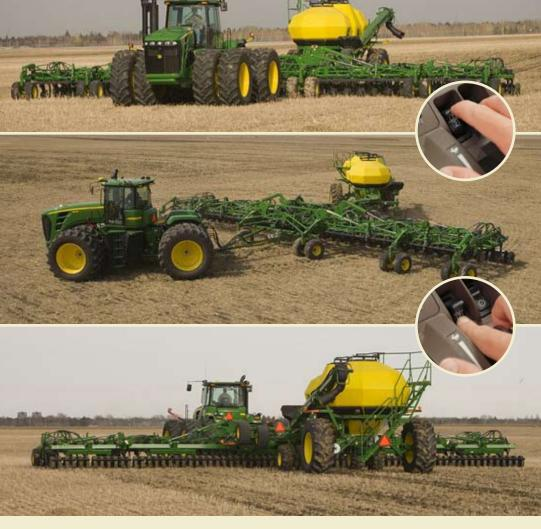
Set the Implement Management System (IMS) to simultaneously perform up to 10 tractor functions per switch (20 total) - push-button easy. You can simplify complicated turn sequences and even less experienced operators can become more productive in less time. IMS boosts efficiency, enhances productivity, and reduces operator fatigue.
