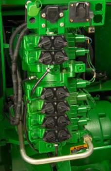
When greater hydraulic capacity is needed up to six SCV remotes are available as a fieldinstalled option.
