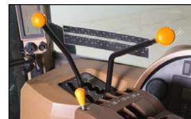
The 24-speed Powr-sync transmission includes a powershiftable hi-lo feature that lets you easily change speeds as field conditions change.
