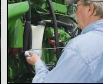
Access to common service check points is unobstructed making daily oil and coolant level checks quick and easy.
