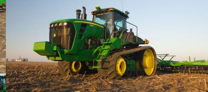
For operations that require the ground-gripping performance and high-flotation capability of a track tractor look no further than a new 9630T. With up to 530 engine horsepower, you can pull large implements like this new 2310 Mulch Finisher, with confidence.
