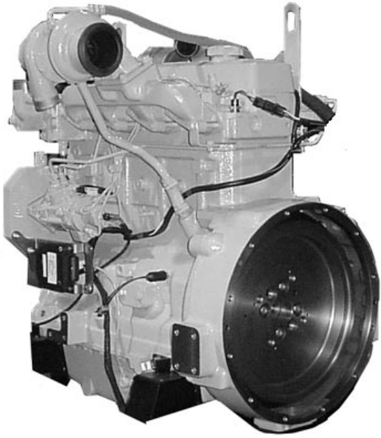
4045 Engine (Stanadyne DE10 Injection Pump Shown)
