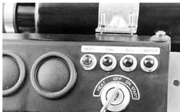
Key Switch in "ON" Position (4.5 L "270" Engines)
