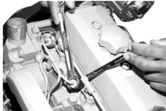
Bleed At Fuel Injection Nozzles
