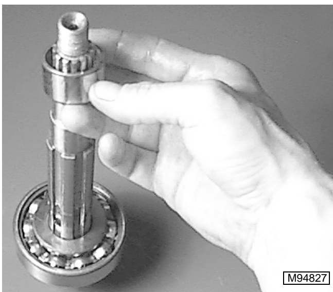
15. Remove 50 tooth gear.
