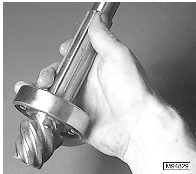
18. Using a suitable puller or press, remove bearing from pinion shaft. Inspect bearing for smooth operation, wear, or damage. Replace as necessary.
