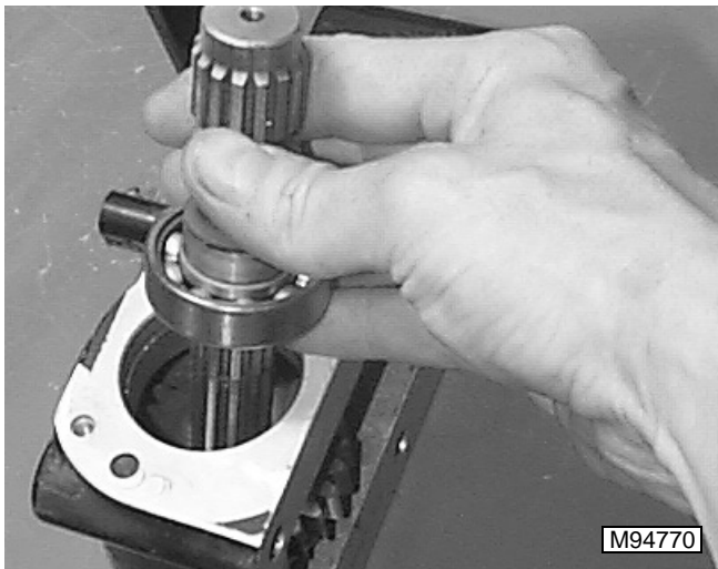
5. Remove shaft and bearing from case as an assembly.
