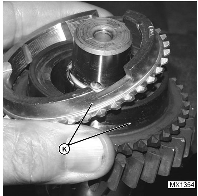
12. Remove gear and brass synchronizer ring (K).
