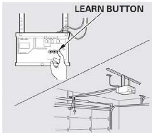
5. Firmly press and release the “learn” or “smart” button. (The name and color of the button may vary by manufacturer.) There are typically 30 seconds to initiate step 6.
