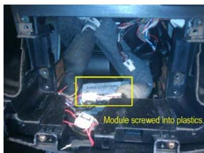
Radio harness is plugged into back of Radio. Radio is mounted into Instrument Panel with 4 screws.
