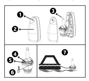
It is not recommended to operate the beacon inside a life raft or under a cover or canopy. Do NOT tie the lanyard to the ship in distress, as this will prevent the unit to functioning if the ship sinks.
