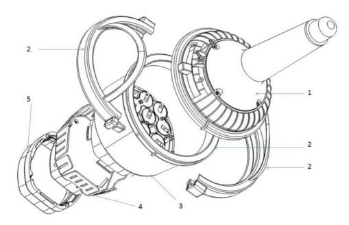
Tron 40VDR Float Free Capsule consists of upper and lower house mounted together with an equator ring. On the lower housing, the VDR storage module is fitted as a removable module, connected to the EPIRB through a clamp.
