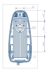
Installation of the FB-40 bracket can be made direct on the ship-wall, as long as the contact of the surface is plane and the areas is bigger than the actual bracket. The FB-40 needs firm ground contact on the grounding screw. Please ensure as short and wide grounding path as possible. Apply silicone grease on the screw before mounting to ensure good connection.
