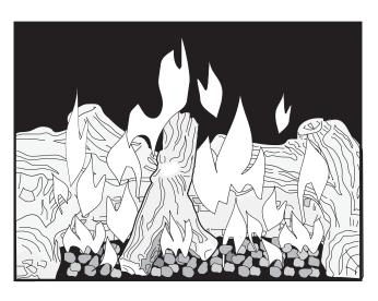
Figure 31. Flame appearance on the "high" setting after approximately 15 to 20 minutes burning.
