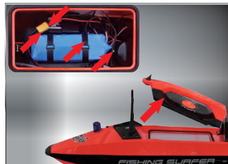
Put battery inside, fix it with velcro strap. Use battery plug to plug in receiver power connector,the light on the receiver turns on ( remarks:The transmitter shall switch on before receiver switch on), then the control system is working.
