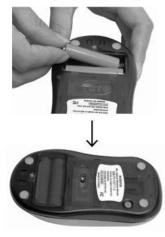
After the AAA Batteries have been installed into your Mouse properly, the sensor LED inside your Mouse will light up.
