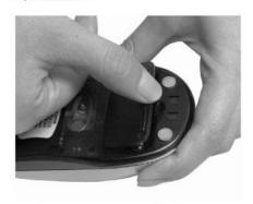
Install two AAA Batteries into your Mouse following the battery orientation guide in the battery bay and then replace the Battery Compartment Cover back onto your Mouse until it securely locks.
