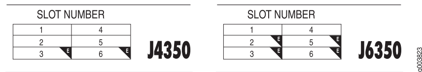
Figure 20: Slot Number Diagram on Front Panel
