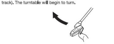
11. Gently lower the TONE ARM by slowly releasing the CUE LEVER. You can lower the TONE ARM manually if the CUE LEVER has not been raised.
