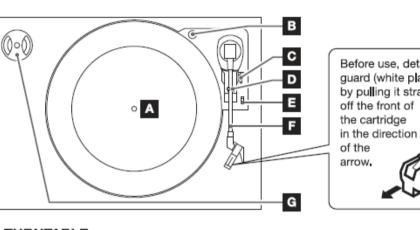
**A** TURNTABLE B TRANSPORTATION SCREW Before use, completely loosen the screw by turning it clockwise with a coin or screwdriver. When you transport the unit, turn the screw counter clockwise to secure the turntable.
