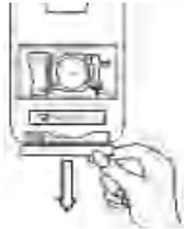
3. Place a new CR2025 battery in the battery holder per the +/- markings displayed on the back of the remote. See Fig. 2.
