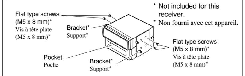
**Note** : When installing the receiver on the mounting bracket, make sure to use the 8 mm-long screws. If longer screws are used, they could damage the receiver.
