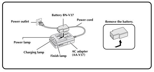
Connect the AC adapter's power cord to a power outlet.
