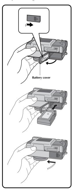
Slide the battery cover slightly to open.
