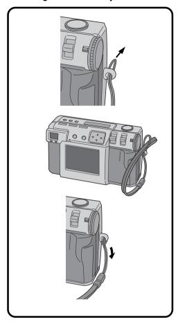
Pass one end of the hand strap through the mounting hole.
