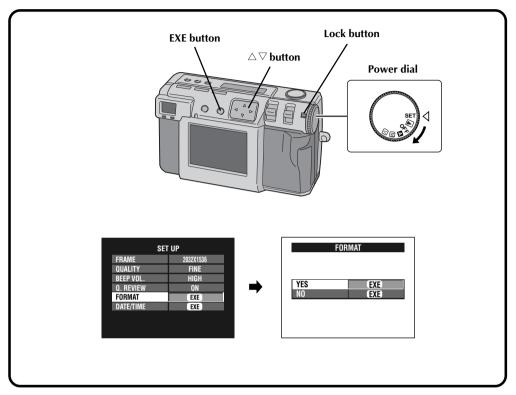
Make sure to use the provided AC adapter (AA-V37) to power the camera, when formatting a Memory card. ( pp. 20)
