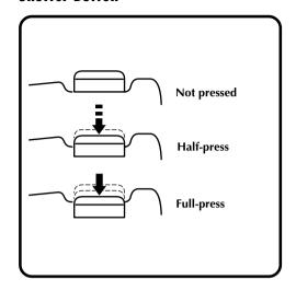
The camera's Shutter button is a two-step button. Pressing it halfway (to the first step) causes the photo standby lamp (green) to flash while the camera focuses automatically.
