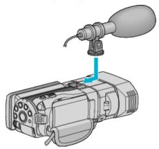
2 Open the cover of the microphone connector and connect the cable of the external microphone.
