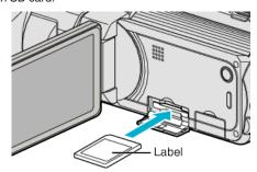
• Insert with the label facing upwards.
