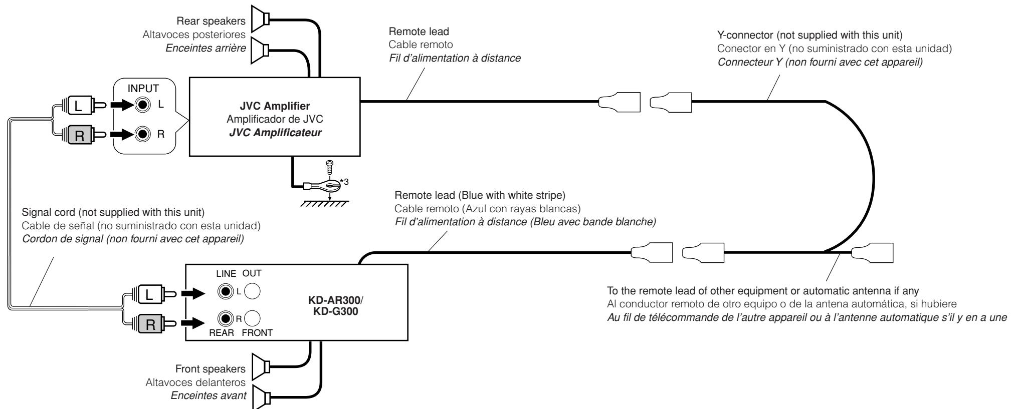
\*<sup>3</sup> Firmly attach the ground wire to the metallic body or to the chassis of the car—to the place not coated with paint (if coated with paint, remove the paint before attaching the wire). Failure to do so may cause damage to the unit.
