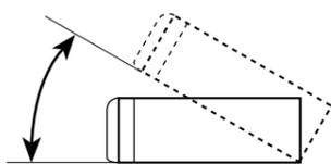
Install the unit at an angle of less than 30°.
