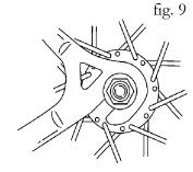
Bolt-on Wheel in Rear Dropoutts
