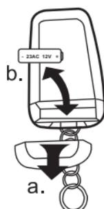
Replace battery when red indicator light 1. does not flicker when a button is pressed. Remove battery cover a. to replace the A23 12V battery b.
