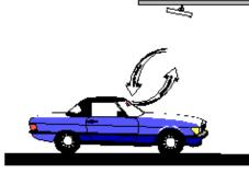
The transponder mosous on the interior sanface of the windshield, behind the rearriew mirror. This maintains a dear view of the road for the driver, and commonicates with automas movested above or alongside the road.
