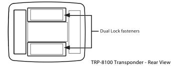
3. Remove the transponder by lifting any corner with sufficient force to separate the Dual Lock strips. Do not reuse the Dual Lock strips if removing them from the windshield. Obtain new strips as required.
