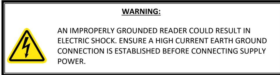
The system integrator supplies the earth ground system for the Reader as per the IEEE 142-2007 standard, particularly; *chapter 5: Sensitive Electronic Equipment Grounding*; and *chapter 3* pertaining to lightning protection; and all other chapter sections describing bonding applications.
