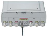
Connect a control cable to the daisy chain input of the FlexRET. The tightening torque for fixing the connector must be  $0.5-1.0~\mathrm{Nm}$  ('hand-tightened').
