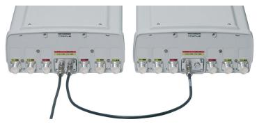
For daisy chain operation, remove the protection cap and attach a control cable to interconnect with the daisy chain input of the subsequent FlexRET or external RCU.
