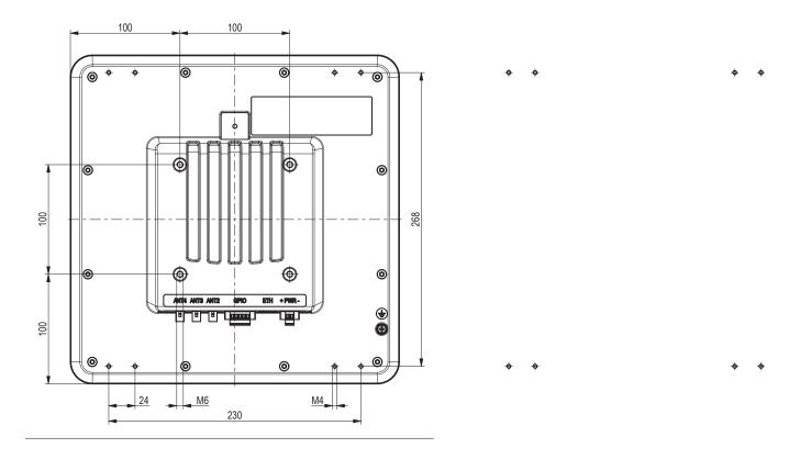
Fig. 12: ARU 2400 dimensions, rear view
