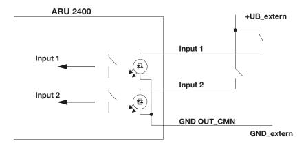
Fig. 19: DC-isolated inputs
