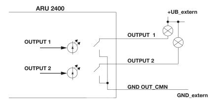
Fig. 20: DC-isolated outputs
