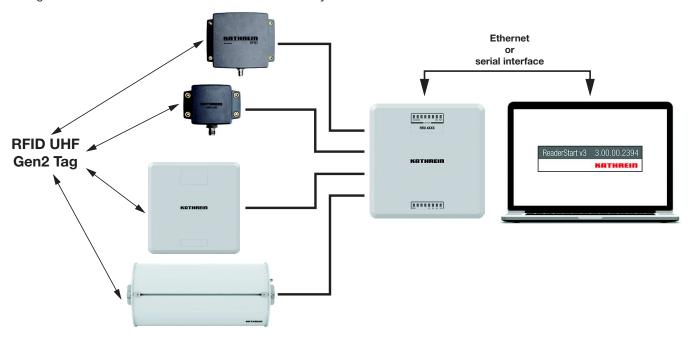
Fig. 1: RFID system (example)
