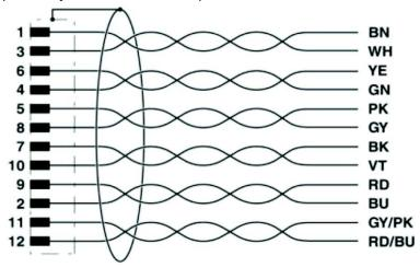
Fig. 13: Allocation of the GPIO interface cable
