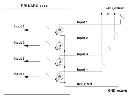
Fig. 14: DC-isolated inputs
