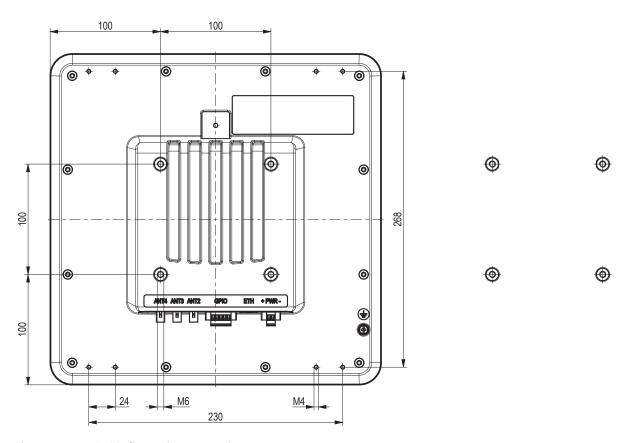
Fig. 11: ARU 2400 dimensions, rear view
