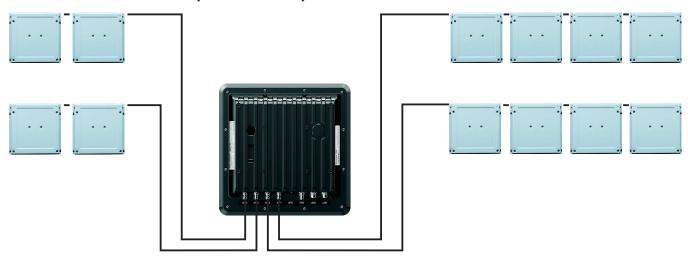
Fig. 4: ©KRAI smart shelf antennas connected to the reader (cascaded)
