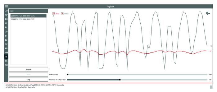
Fig. 78: TagScan: phase shift, transponder is moved
