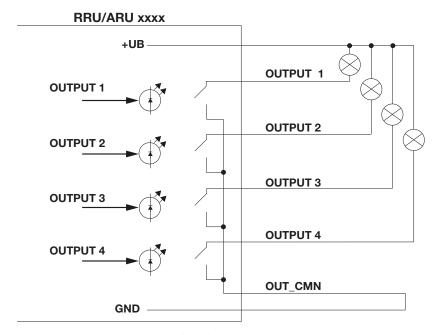
Fig. 17: Outputs, not DC-isolated
