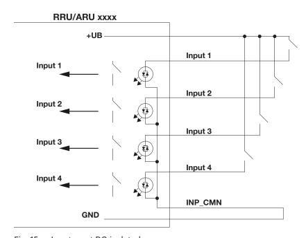
Fig. 15: Inputs, not DC-isolated
