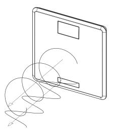
Fig. 3: Circular and linear polarisation
