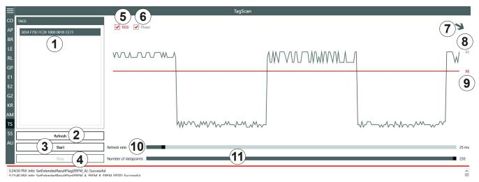
Fig. 77: TagScan: phase shift (due to the channel change), transponder is not moved
