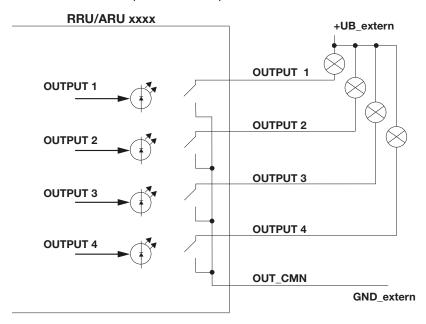
Fig. 16: DC-isolated outputs
