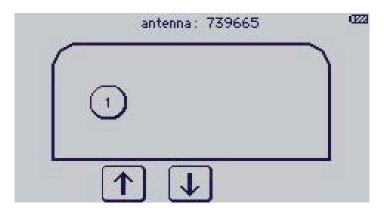
You must click on a port (1, 2, ...) to open a new display view. In this view you will see a list of RETs from which you can select the corresponding and RET and confirm by pressing 'Select Ret'.
