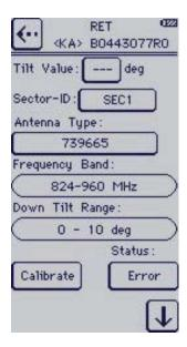
The 'Tilt Value' button opens an entry for a new tilt value.
