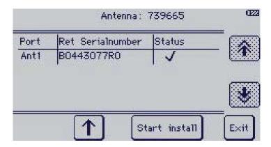
Push the button 'Start Install' to start automatic installation of the assigned RETs.
