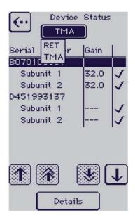
In this view, the individal ALDs are listed separately for RET and TMA. Click the button 'RET' to view a dropdown list where you can choose between RET and TMA. The units will be listed according to your selection. Use the arrows located under the list to navigate through the list. Select a unit and then click on the button 'Details' to change over to the detailed view.
