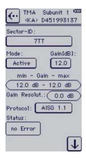
When the TMA has variable gain values, the gain value must be selected.
