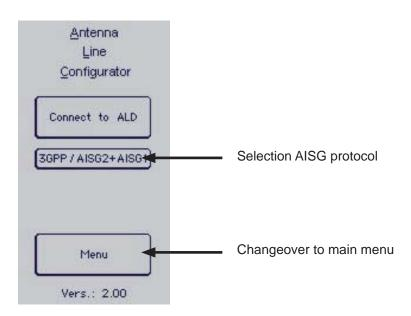
The start screen will appear after the unit has been booted. One can set the AISG protocol for the set-up of the connection here.
