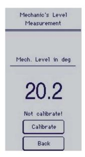
To calibrate the sensor, hold the ALC on a vertical object and press the button 'Calibrate'. Stop the ALC, press the button 'Calibrate' and the device is calibrated.
