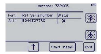
When the calibration wizard is finished, a status symbol will appear on each RET. To leave the installation wizard and return to the main menu, press the 'Exit' button.
