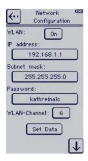
WLAN can be switched on or off as desired. The IP address and the subnet mask can be set. The WLAN password is preset and can be changed over the button 'Password'. The WLAN channel can be set between Channel 2 and 11.
