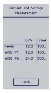
Displays electricity and voltage values on the feeder cable and AISG bus
