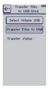
Use the button 'Select Volume USB' to select the USB stick. Now press the button 'Transfer File to USB'. All Report Files will be transferred from the ALC to the USB stick.
