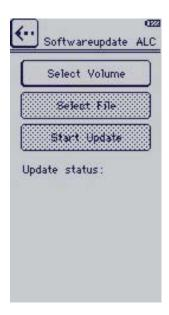
To update, select the partition on the memory stick. Afterwards, select the file using the 'Select File' button. Press 'Start Update' to start the installation procedure. This may take several minutes.
