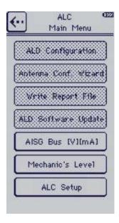
Press the button 'ALD Configuration' to access the view in which the ALDs are listed divided into the categories RET and TMA.
