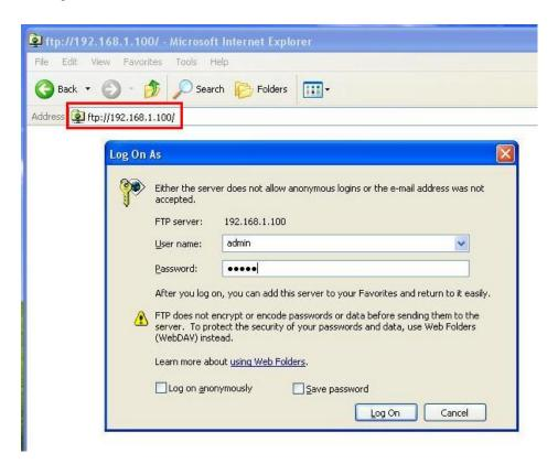
Open Internet browser and input the address of the router. For example, we use <a href="ftp://192.168.1.100">ftp://192.168.1.100</a> because the LAN IP address of our router is 192.168.1.100.
