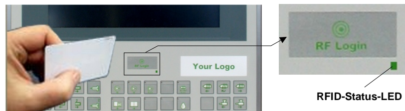
Contactless user identification with an RFID card (e.g. operating panel)
