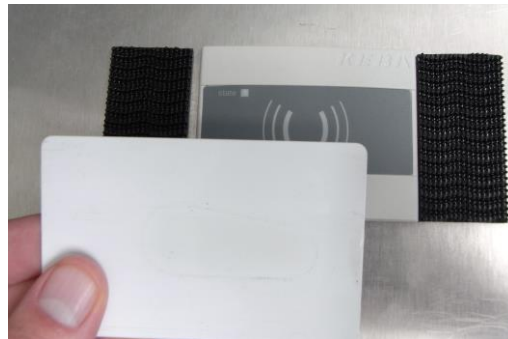
Contactless user identification with an RFID card (e.g. operating panel)
