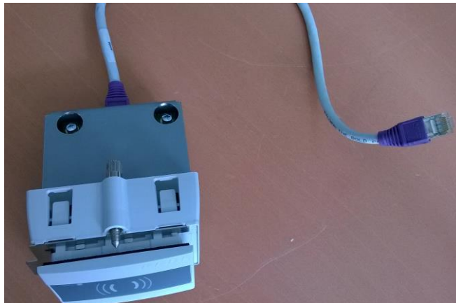
RFID module after installation
