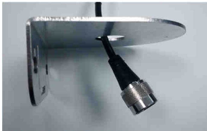
Figure 74 : N connector introduced in the hole of the dome antenna bracket
