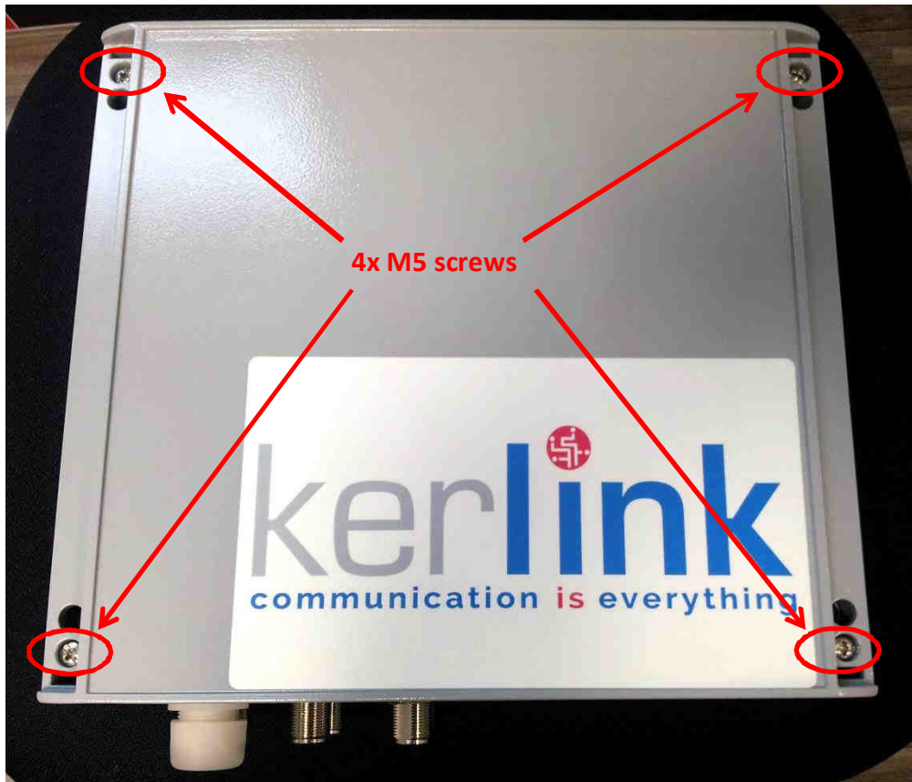
Figure 62: Wirnet iBTS – 4x M5 screws
