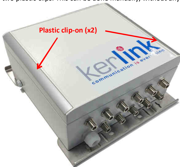
Figure 61: Wirnet iBTS – plastic clips on the lid
