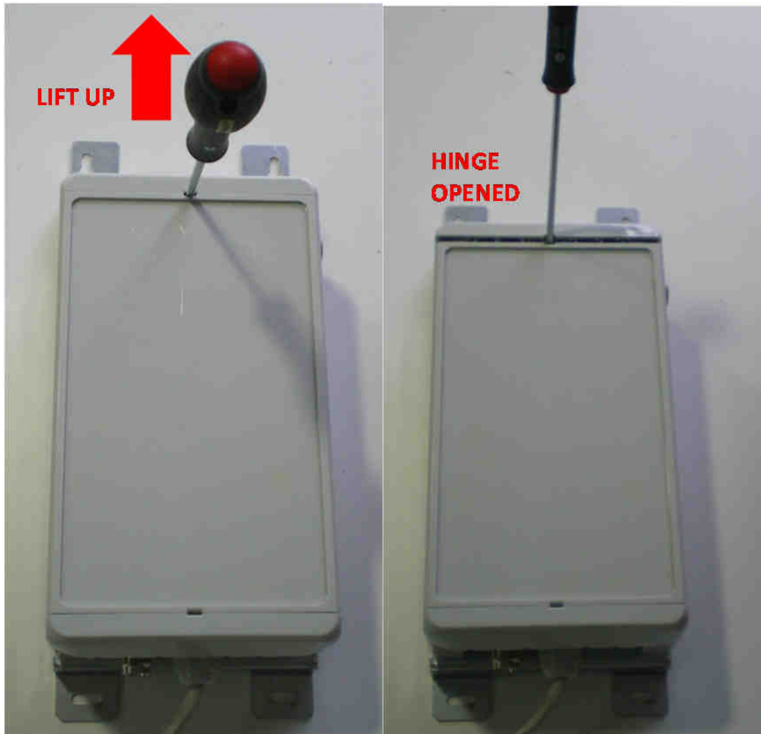
Figure 64 : Opening of the compact enclosure with screwdriver
