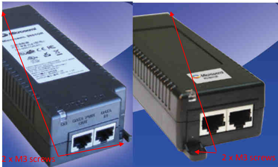
Figure 87 : Screws for indoor POE injectors mounting
