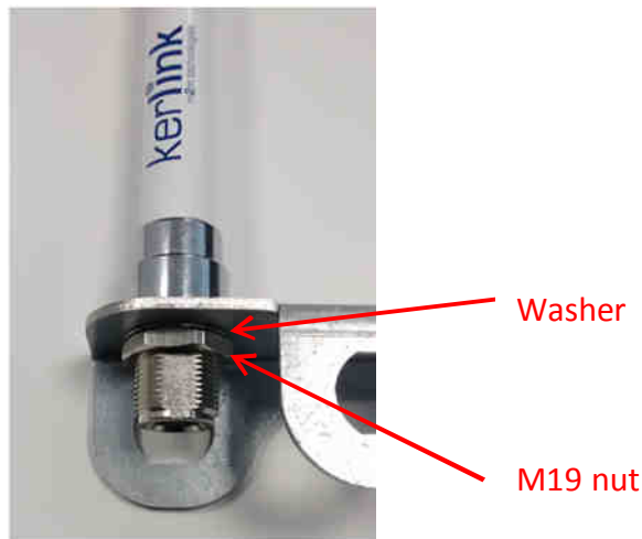
Figure 73 : LoRa antenna mounted on universal antenna bracket
