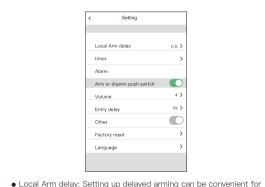
users to go out in the case of time buffer (delayed trigger detect gateway will not alarm), 0-255 seconds can be set; • Timer: Users can set up timed arming and disarming and alarming according to their needs Arm or disarm push switch: After opening the arming and disarming
