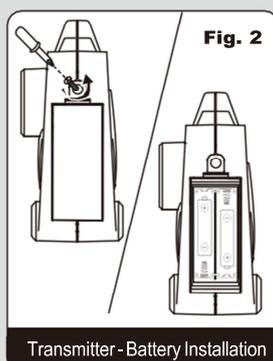
Transmitter - Battery Installation
