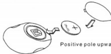
Positive pole upwards to install the battery.
