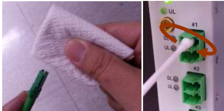
Figure 3-3 Optic Connector Cleaning (left) and Optic Port Cleaning (right)
