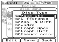
For example, when the screen shows the guidance <code>Edit</code> <code>Save</code> <code>Back</code>, the <code>[SAMPLE]</code>, <code>[SAVE/SEL]</code> and <code>[TARGET]</code> buttons are assigned with the Edit, Save and Back functions respectively. In this manual, when the button name and the function assigned to the button are different, the button name and function are described as "the <code>[SAMPLE]</code> (Edit) button" or "<code>[TARGET]</code> (Back) button".
