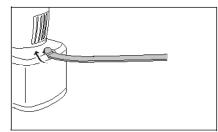
Pass other end of Wrist Strap through the ring, and pass the strap that passed through the strap holder through the ring too.
