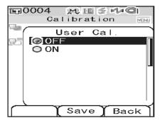
3 Use the ∇ button of the cross key to move the cursor to "ON" and then press the [SAVE/SEL] button.
