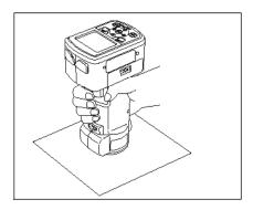
4 Make sure that **€** (Ready to measure) is displayed or Ready lamp is green, and then press the measuring button.
