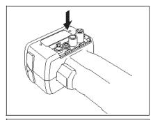
Align the grooves of the cover with the guides on the edge of the battery chamber opening. Press down lightly on the cover and slide it upward to close it.
