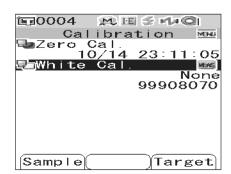
3 If necessary, use the ∇ button of the cross key to move the cursor to "White Cal."
