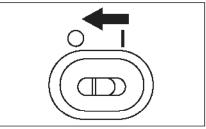
2 Open the connector protection cover of the AC adapter terminal on the instrument.
