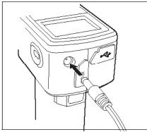
Insert the AC adapter power plug to an AC outlet (100 to 240 VAC, 50-60 Hz).
