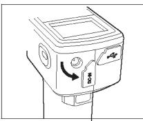
3 Connect the AC adapter connector jack to the AC adapter terminal.
