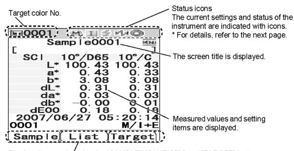
The functions assigned to the [SAMPLE], [SAVE/SEL] and [TARGET] buttons are displayed respectively.
