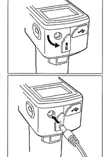
Insert the AC adapter power plug to an AC outlet (100 to 240 VAC, 50-60 Hz).
