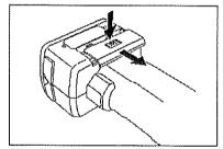
Place four AA-size batteries in the battery chamber. Make sure that the batteries are placed in the correct direction.
