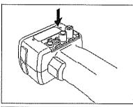
Align the grooves of the cover with the guides on the edge of the battery chamber opening. Press down lightly on the cover and slide it upward to close it.
