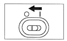
Press the battery chamber cover button on the side of the instrument and slide the cover downward to open it.
