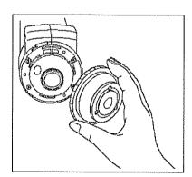
2. Use a blower to remove dirt and dust from the integrating sphere.
