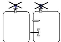
**Do not** position in tank **centerline**! (multiple reflections!)
