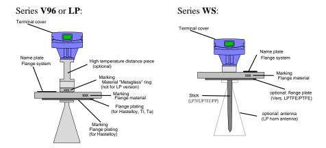
Marking of the **signal converter** (see name plate):
