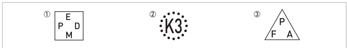
Figure 2-7: Symbols for the supplied gasket material (on the side of the process connection)
